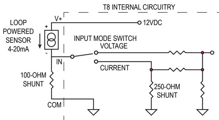
Connect external 100-ohm shunt between input and common (gnd) terminal.
